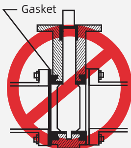
Figure 3 - Initial Centering & Flanging of Valve.
